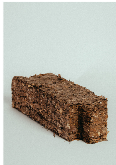
Interlocking insulation blocks made from leaves and resin. The notch allows the block to fit inbetween the studs.
