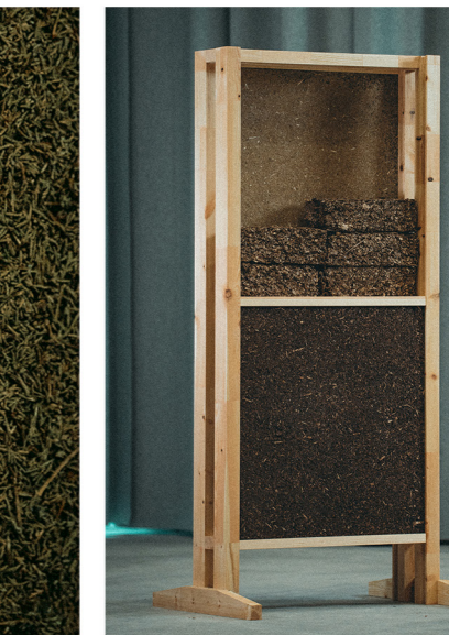
View of the exterior panel (Top panel is removed for view into leaf insulation)
